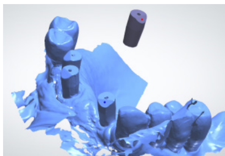
5. In the 3Shape Dental Designer at the dental laboratory the Elos Accurate IO Scan Body was aligning the material file from the Elos Accurate Library.
